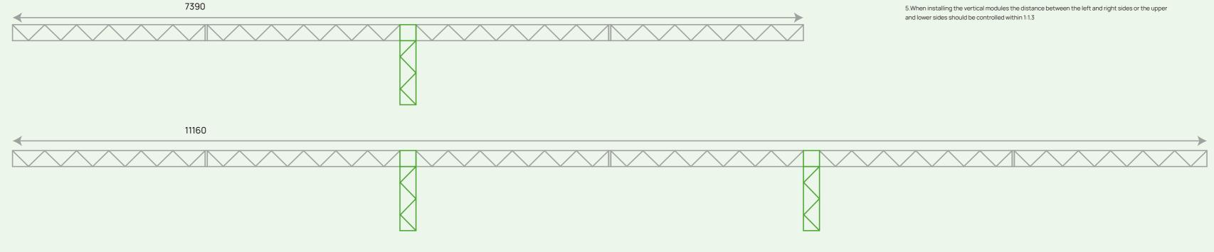
3.When length a≤3620mm do not need to connect with corner block or vertical module, 3620 < a ≤7390 need to add one corner block and vertical module,,7370 < a≤11160 nned to add two corner blocks and vertical module, and so on
