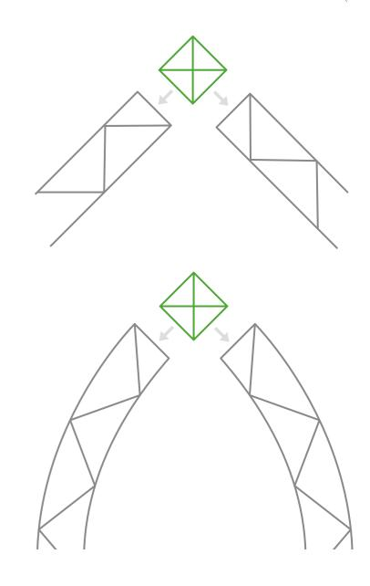
2.The connection of the corner part only can use the corner block to connect
