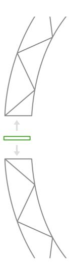
1.Corner block and connecting cross can be used for connection between straight/curved sections, but corner block is preferred
