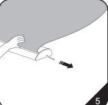
5. Hold the graphic and remove the pin
