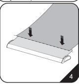
4. Peel off the adhesive paper along the edge of the base's leader roll and attach the bottom of the banner. Make sure the banner is straight.
