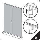
8. Lift the graphic and make it fixed onto top of the pole.
