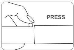
If can't snap when dismantle the frame, Pls push the tube forwardly, then push again.
