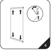
4.Open the clip snap bar then insert both edge of the graphic.
