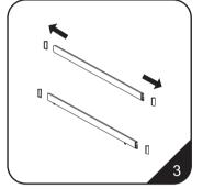
3. Remove the plastic end caps from the clip bar.
