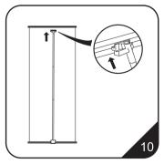
10.The plastic holder at the top of pole slips into the rear slot of the banner beam. A marker on the beam indicated the beam's centre where the pole should be inserted.
