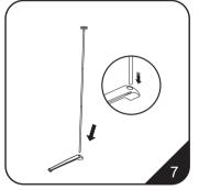
7. Insert the assembled pole into the base hole.
