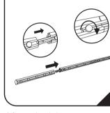
3.Connect the rails by screws.
