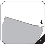
4.Remove the double side glue in the insert quickset, stick 4 of them to the backside four sides of the grahic.
