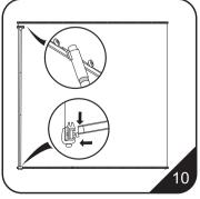
10. Assemble the vertical pole with the top rails (Notice:make sure the rails with adjusting screw
